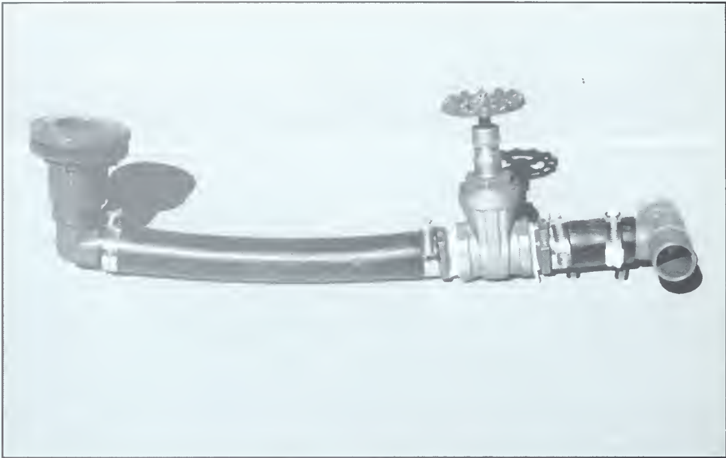
Photo 4. Tank plumbing assembly, left to right: bulkhead fastener, 90° MIP-plastic barbed adapter, polypipe with hose clamps, MIP-barbed adapter, brass gate valve, MIP-barbed adapter, polypipe with hose clamps, plastic tee.
